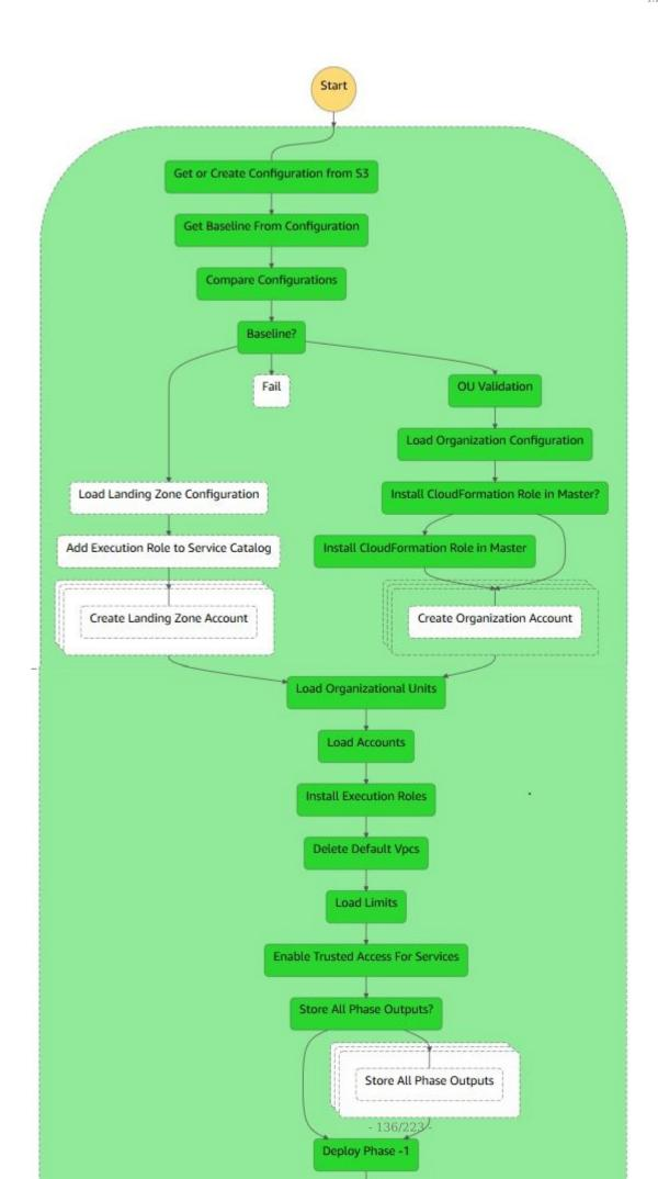
Notice the extremely linear state machine design. This was done to reduce complexity and ease troubleshooting. You may notice a small fork in the state machine. The left path is executed if the Accelerator is deployed on top of an ALZ, The right path is executed if the Accelerator is deployed as a standalone solution. If we eventually add a Control Tower deployment option, it is likely it could also leverage the existing ALZ path.
