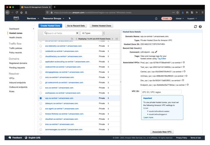
From within an associated workload VPC such as <code>Dev</code>, the service endpoint (e.g. <code>sqs.ca-central-1.amazonaws.com</code>) will resolve to an IP in the <code>Endpoint VPC</code>:
