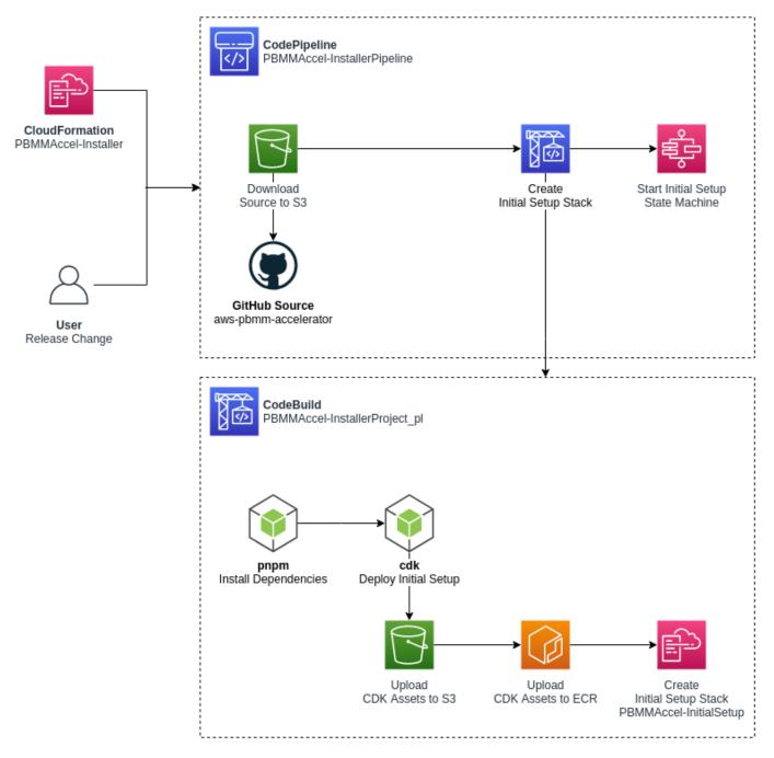
The ASEA-InstallerPipeline starts when first installed using the CloudFormation template. The administrator can also start the pipeline manually by clicking the Release Change button in the AWS Console.
