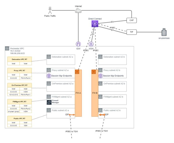
This VPC has four subnets per AZ, each of which hosts a port used by the NGFW devices, which are deployed in an HA pair. The purpose of these subnets is as follows.
